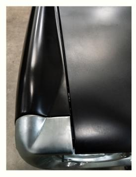
Any new Bronco body tub requires final finishing if it is intended to be more than a driver. An experienced restoration body shop must spend considerable hours massaging the metal before they can begin surfacing. Specializing in this work allows Agaso to help clients mitigate additional costs with their body shop by having the body well gapped upon delivery.
