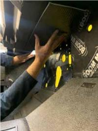
**Step 4:** Remove backing on boom mat layer pieces and install on firewall. Optional: use roller to final mount material and maximize adhesion. Recommend gloves as edges can be sharp.
